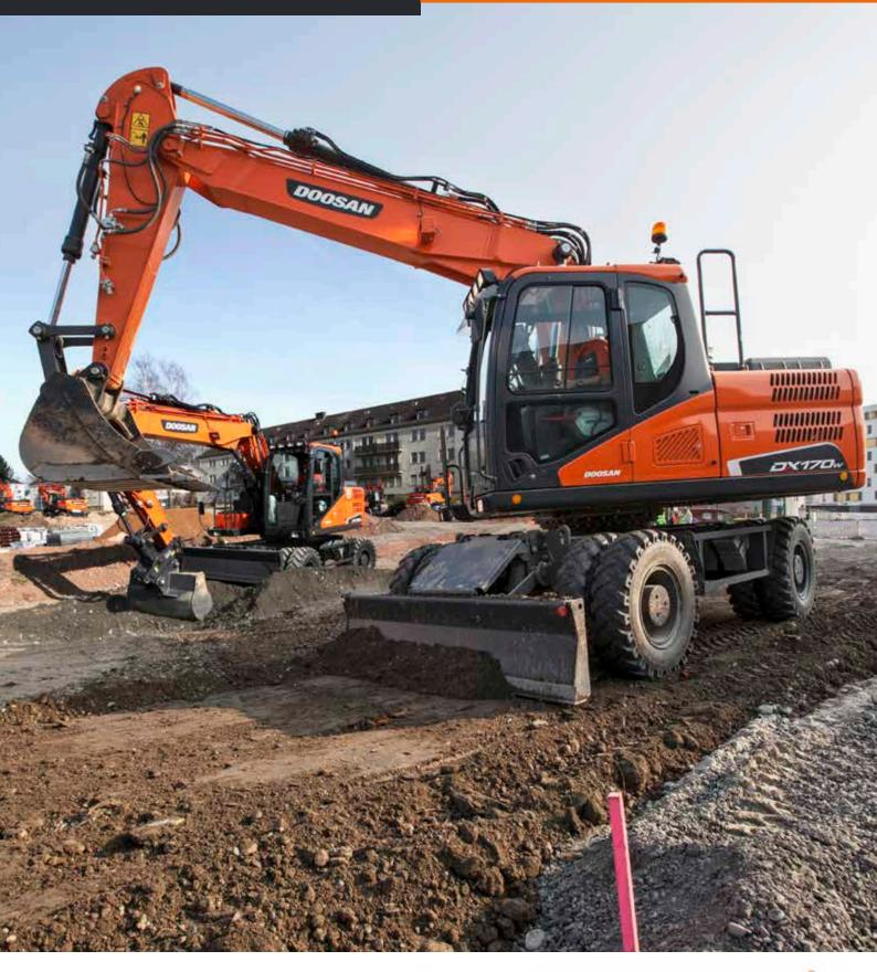
Maximum power: 152 hp Operating weight: 16.8 t Max. bucket capacity: 0.90 m³
