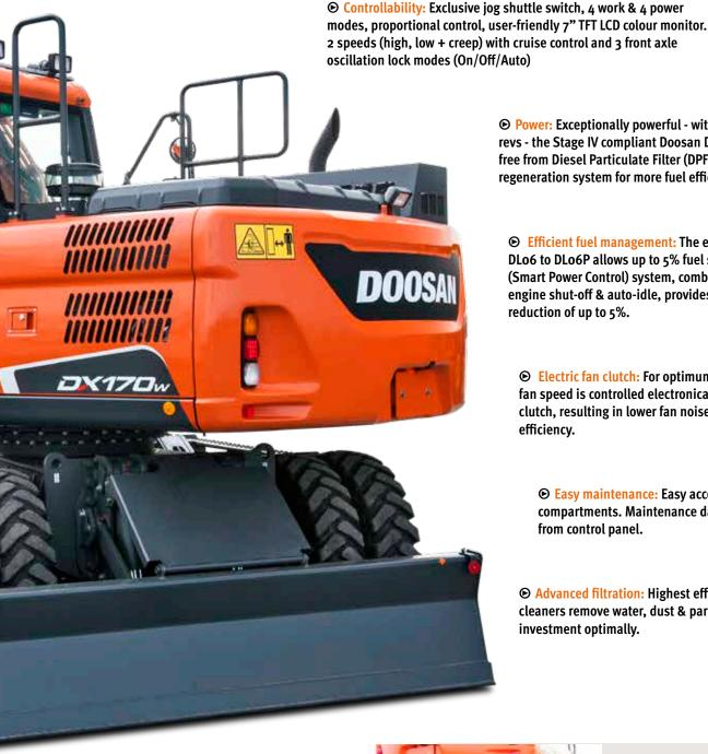
**Power:** Exceptionally powerful - with high torque at low revs - the Stage IV compliant Doosan DLo6P engines are free from Diesel Particulate Filter (DPF) and associated regeneration system for more fuel efficiency.
